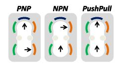
The alternate flashing of the LED "Red" and "*Green*" confirms the new outputs configuration. At this stage, it is requested to position both the trimmers in *RUN* mode.
