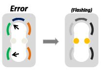
In this case the sensor waits that the end user positions both the trimmers in RUN mode or it is requested to switch off the sensor and repeat properly the product configuration.
